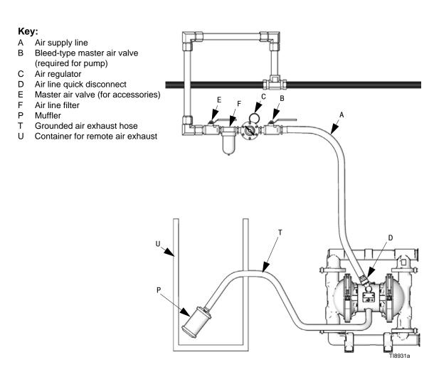
Fig. 4 Venting Exhaust Air
