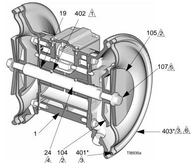
Cutaway view, with diaphragms in place 24 <u>4</u> 2 <u> 3</u> 24 🐴 104 🖄 401\* 🖄 🙆 403\* 🖄 105 🖄
