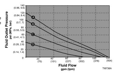
AIR PRESSURES A = @ 120 psi (8.4 bar, 0.84 MPa) (B) = @ 100 psi (7.0 bar, 0.7 MPa) ©= @ 70 psi (4.8 bar, 0.5 MPa) D = @ 40 psi (2.8 bar, 0.3 MPa)
