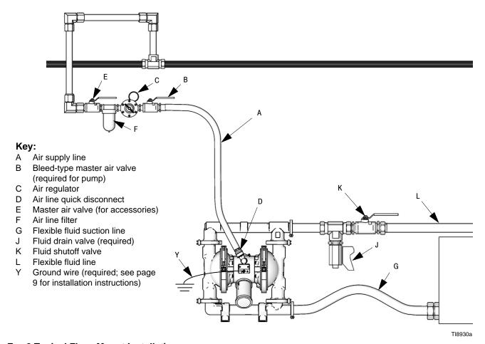
Fig. 2 Typical Floor-Mount Installation
